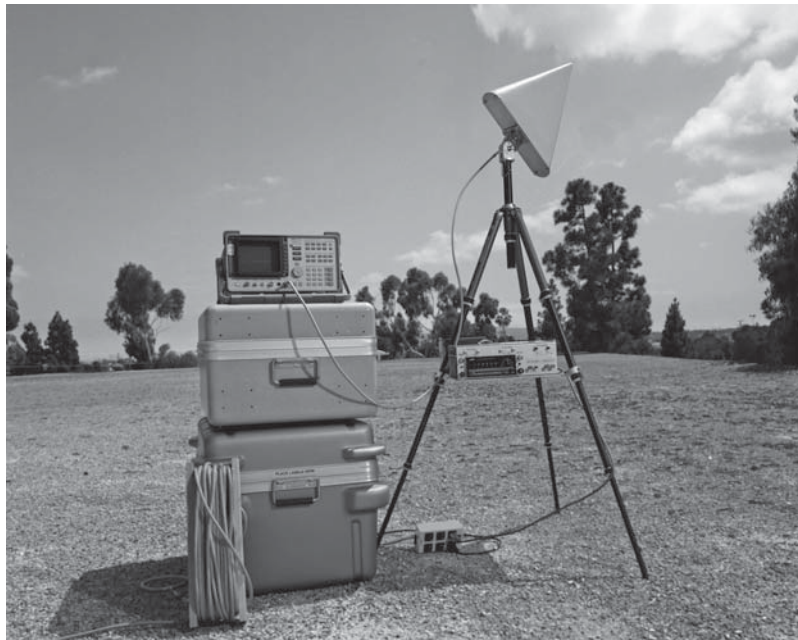
Figure 5-2 RF site survey equipment [1]
